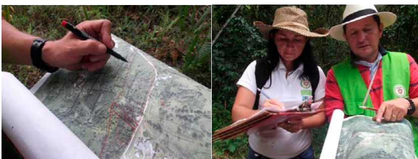
▲ Figure 1, Fit-for-purpose land administration. Identified boundaries are drawn in the field on top of an orthophoto (left), while administrative data is recorded simultaneously (right).
