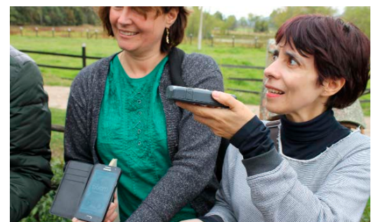
▲ Figure 2, The Trimble R1 has a Bluetooth connection with a mobile on which also Esri's Collector App is installed.
