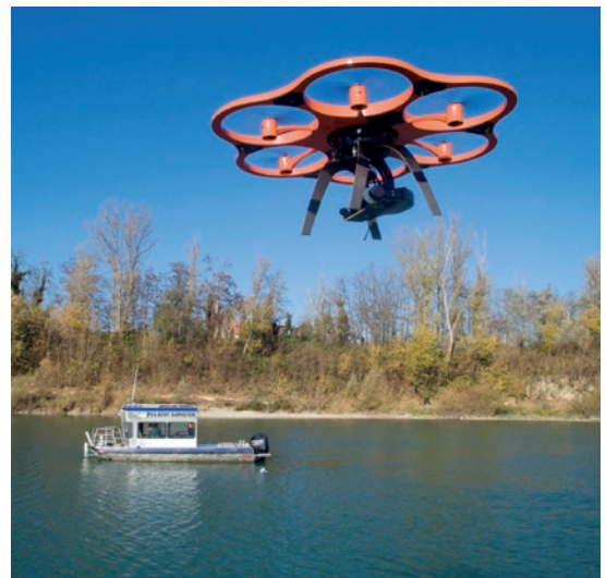
▲ Figure 1, Simultaneous hydrographic and air survey.
