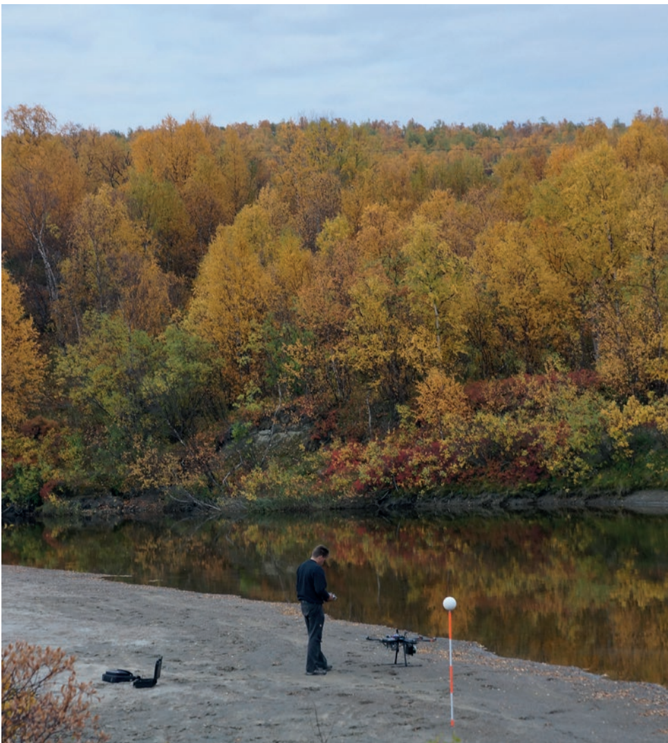
▲ Figure 1, Launching a small UAS for a topographic laser scanning mission in the Finnish Arctic. Multi-temporal laser scanning data is collected to monitor Arctic river bed morphology.
