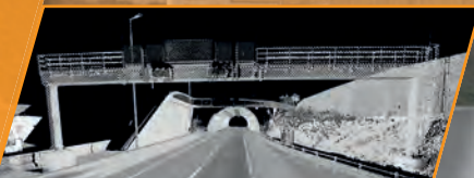
Infrastructure Mapping (VMX-1HA scan data acquired in a single pass)
