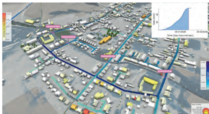
▲ Figure 4: Storm water scenario in an Austrian town. Water depth in sewer pipes is colour-coded.
