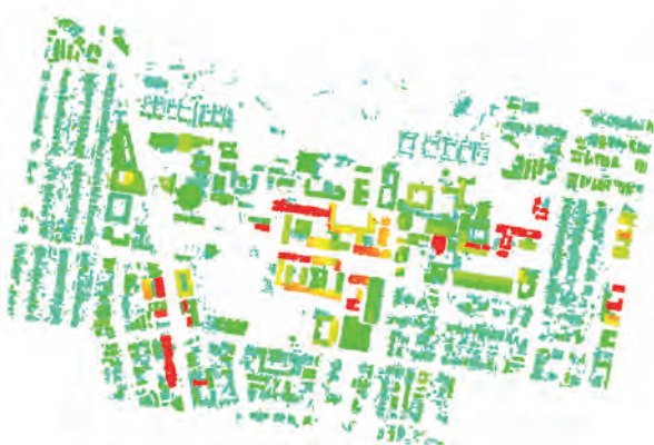
▲ Figure 4: Building points extracted from 2005 Lidar data and classified by object-based methods in ERDAS.
