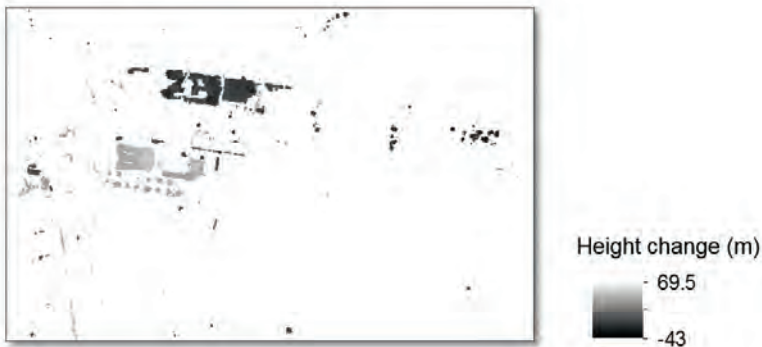
▲ Figure 6: The results from the new solution combining a machine learning algorithm with DSM differencing.
