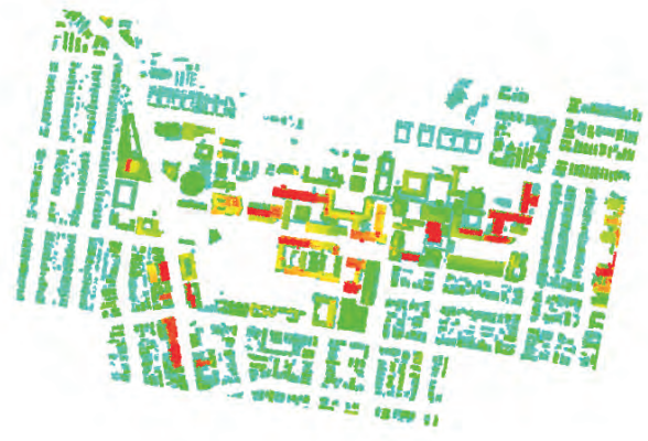
▲ Figure 5: Building points extracted from 2008 Lidar data and classified by object-based methods in ERDAS.
