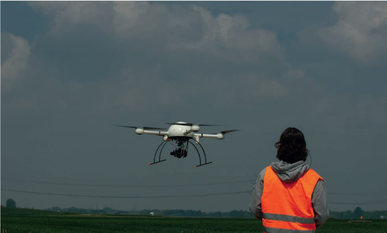
▲ Figure 3, A quadcopter UAV equipped with camera to map crop differences.
