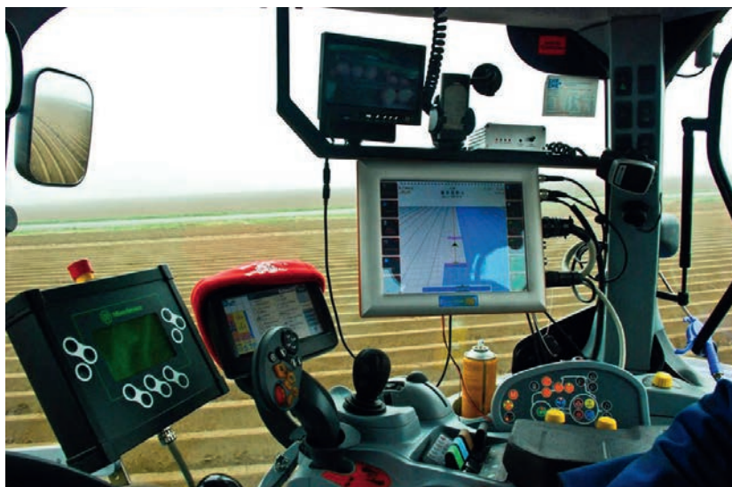
▲ Figure 1, The tractor 'cockpit' nowadays is full of screens to help the farmer with steering and location-specific application.
