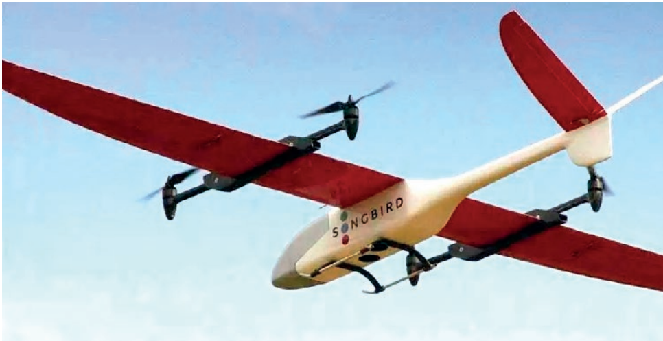
▲ Figure 4, Looking like a fixed wing, this hybrid UAS combines the pros of a fixed wing with the VTOL ability of a copter. (Courtesy: Aerolution)
