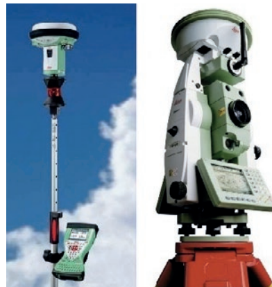
◀ Figure 2, Pole equipped with external controller, prism and GNSS (left) and GNSS antenna on top of total station. (Courtesy: Leica Geosystems)
