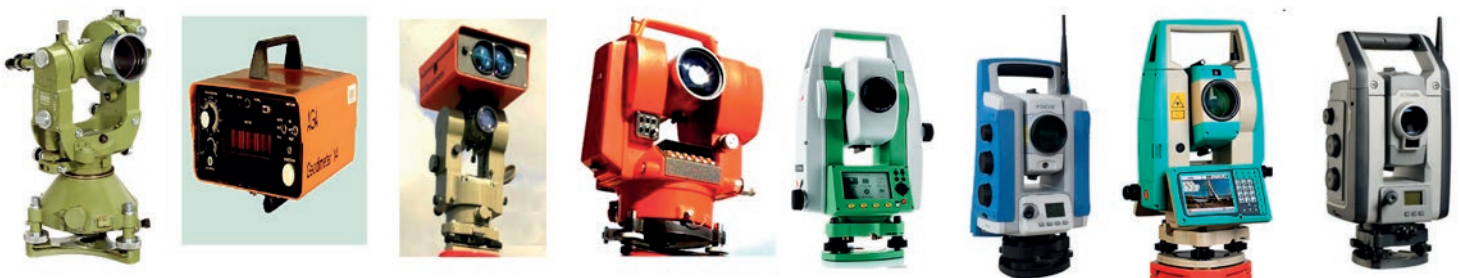
▲ Figure 1, Evolution from theodolite to total station. From left to right: Wild T3, introduced 1925; Aga Geodimeter 14, manufactured 1970; EDM mounted on theodolite, HP 3820A; Leica FlexLine TS02plus (2013); Spectra Precision Focus 35 (2014); Ruide RIS and Trimble S9, both from 2015. (Courtesy: M. Lemmens)
